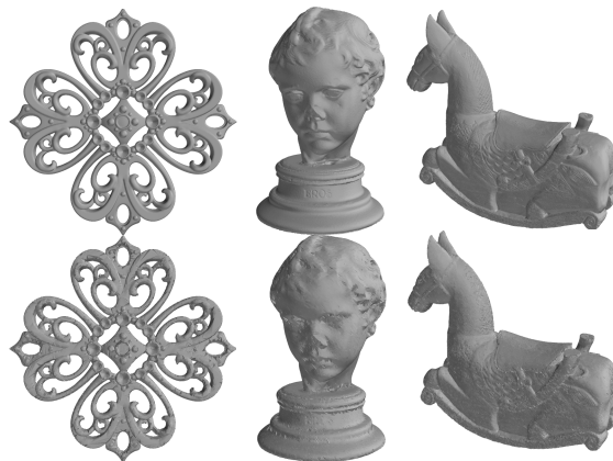
Figure 15: The original Filigree dataset (top left 3.1 million simplices), the contracted Filigree dataset (bottom left - 400,000 simplices), the original Eros dataset (top center - 2.8 million simplices), the contracted Eros dataset (bottom center - 100,000 simplices), the original Isidore dataset (top right - 6.6 million simplices), and the contracted Isidore dataset (bottom right - 1.1 million simplices).
